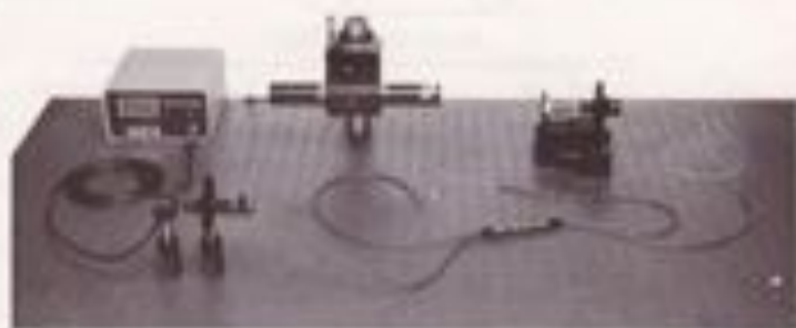
Figure 7.6. Laboratory set-up for studying the bidirectional coupler.
