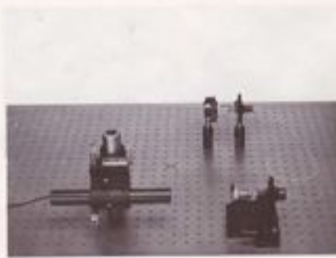
Figure 4.3. Laboratory set-up for observing low order modes in a multimode fiber with low V-number.
