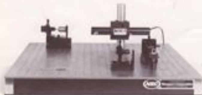
Figure 10.2. Laboratory set-up of the Mach-Zehnder interferometer.
