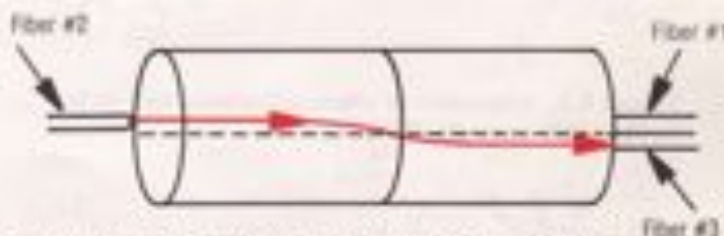
Figure 7.11. Coupling light from fiber #2 to fiber #3. Fiber #2 is placed symmetrically across the center line of the lens from fiber #3 at the opposite end of the lens assembly.
