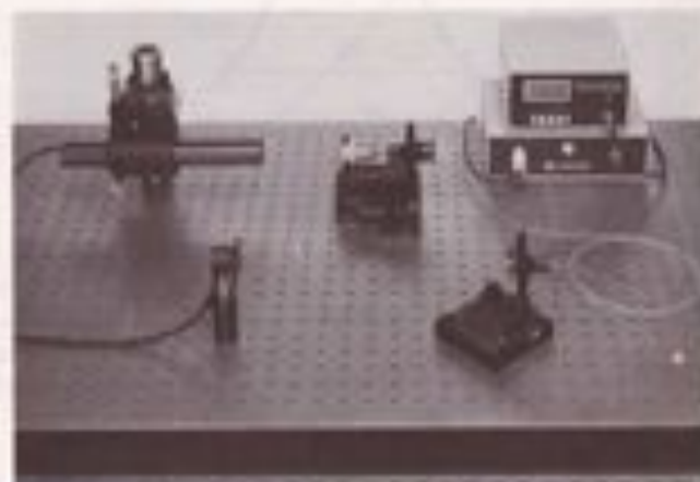
Figure 3.7. Laboratory set-up for examining the Gaussian approximation for a single-mode fiber.
