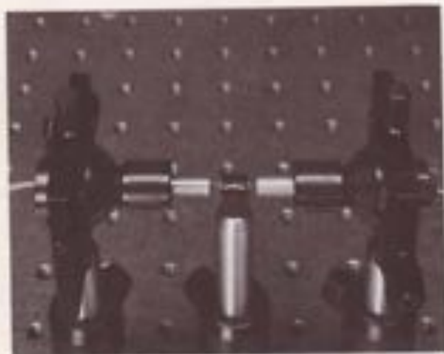
Figure 7.9. Construction of the WDM device. Arrangement of the components is in an orientation which agrees with that shown schematically in Fig. 7.4a.
