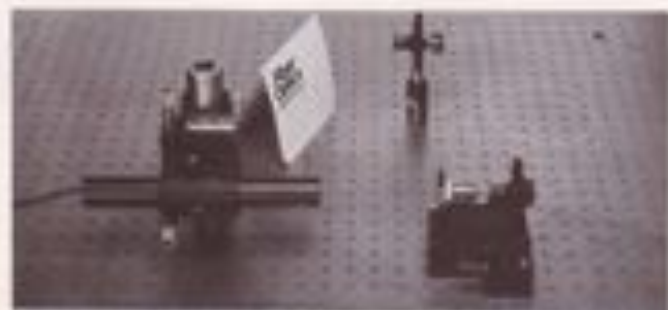
Figure 4.4. Laboratory set-up for orienting the polarization axes of the polarization fiber with the graduations on the chuck from the F-916 Fiber Coupler.
