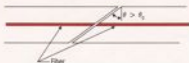
Figure 9.1. Liquid level sensor, \theta_c is the critical angle for total internal reflection at a glass-air interface in the glass fiber.
