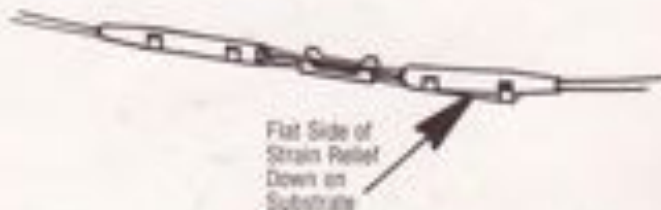
Figure 6.19. Placing strain reliefs on the alignment guide substrate.
